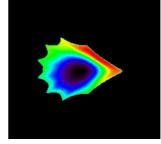
Figure 4: Tomographic reconstruction in the triangular plane of radiated power in a 1 MW NBI partially detached divertor plasma with B = 2.5 T in hydrogen.
