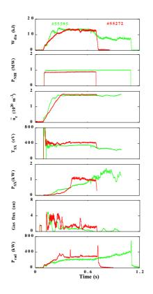
Figure 1: Time evolution of plasma parameters in a 1 MW NBI divertor discharge in hydrogen (green) and deuterium (red) with B = 2.5 T at a density in the vicinity of the density threshold for transition to the high density H-mode.
