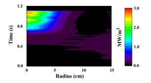
Figure 2: Time evolution of radial profiles of radiated power in a 1 MW NBI divertor plasma at the density threshold with B = 2.5 Tin hydrogen. See #55595 in Fig. 1.
