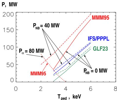
Fig. 1. Influence of the boundary temperature on the power in  $\alpha$ -particles,  $P_\alpha$ , for three different transport models. Solid curves show the case without additional heating, dashed curves show the case with 40 MW of NB heating. Dotted line shows the power of additional heating required for keeping the constant level of  $P_\alpha = 80 \text{ MW}$ . For this case, the left scale shows  $P_{NB}$ .
