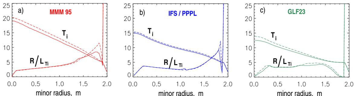
Fig. 2. Profiles of the ion temperature at the same boundary condition  $T_{ped} = 5$  keV for different transport models. Radial dependencies of the dimensionless parameter  $R/L_{Ti}$  are also shown. The temperature is given in keV. The cases with (40 MW) and without additional heating are shown with dashed and solid lines, respectively.
