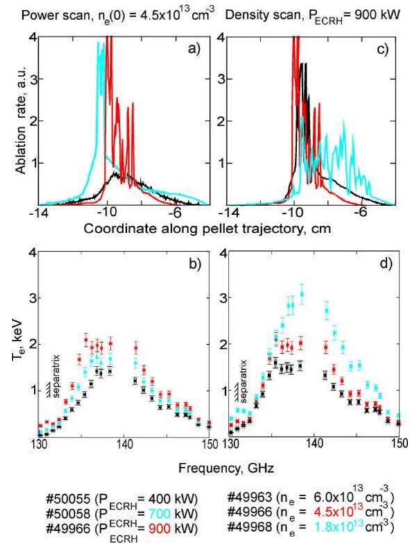
Fig. 1. Ablation rates (upper part) and the ECE signals (lower part) for the power and density scans.
