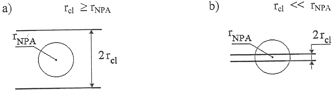
Fig. 16. Possible disposition of a pellet cloud and the area visible to the NPA.
