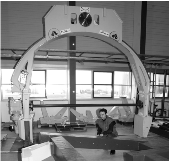
FIG. 3: Coil-handling unit during tests using a coil dummy
