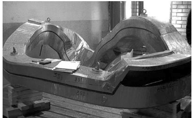
FIG. 1: Two half-shells of a non-planar coil casing during final inspection (by courtesy of BNN)
