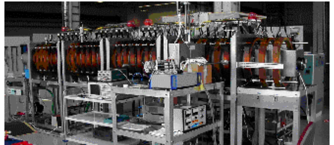
the axis. On the right-hand side, the helicon plasma source is installed.
