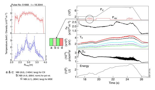
**Figure 1.** On the right, typical time traces of ICRF and NI power, plasma density and temperature,  $D_{\alpha}$  signal and plasma energy. In the sequence of beam blips, the first and third (a and c) in each series of 4 blips, is used to measure the toroidal rotation. On the left, profiles of the density (top) and of the temperature (bottom).
