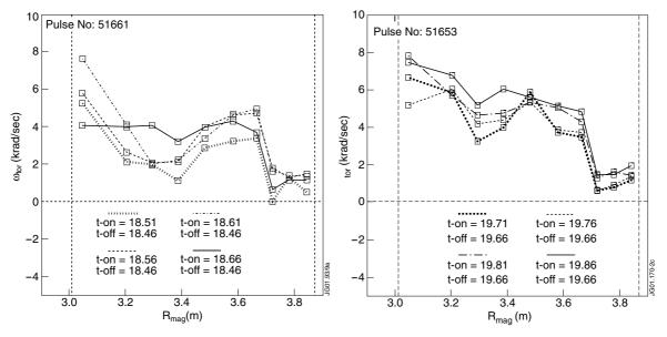
**Figure 2**. On the left (a), rotation profile for a location of the resonance layer at R = 2.5 m,  $P_{IC} = 2.85$  MW, on the right (b) for a location of the resonance layer at R = 2.65 m,  $P_{IC} = 2.9$  MW. In both cases the plasma was in the L-mode. Four rotation profiles taken during a time interval of 200 ms are show. As discussed in the text, the first profile is not markedly influenced by the momentum input of the beam.
