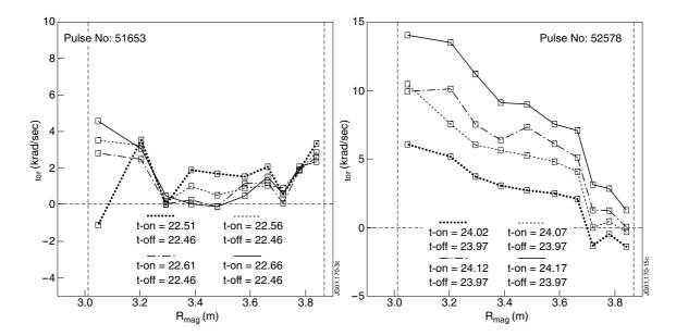
**Figure 3**. Toroidal rotation profile for the same discharge as fig 2b, at a later time, R = 2.95 m,  $P_{IC} = 2.9 \text{ MW}$ , after a period of sawtooth stabilization and subsequent large sawtooth crash.
