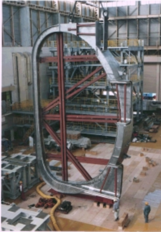
Figure VI: Photograph of the prototype sector of the vacuum vessel for ITER (Photo ITER).
