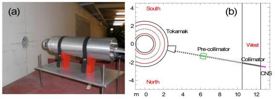
Fig. 2: (Color online) In (a), the CNS installed at AUG in front of the 2-m long neutron collimator obtained in the concrete wall. In (b), schematics of the CNS line of sight from above. The CNS is viewing the plasma radially in the tokamak equatorial plane at a distance of about 11 m from the plasma center through a pre-collimator and a collimator.
