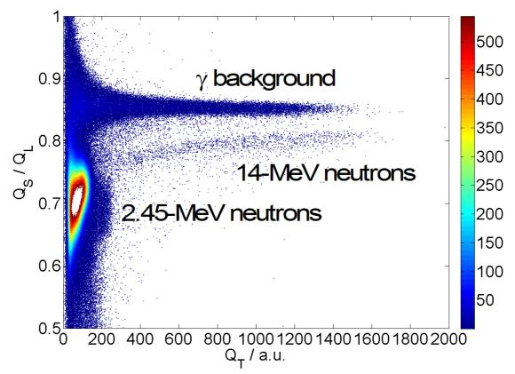
Fig. 8: (Color online) Contour plot of the radiation events recorded in AUG discharge 24151. The pulse shapes were offset reduced and LED corrected and analyzed using the optimal gates S = 4 samples and L = 15 samples.
