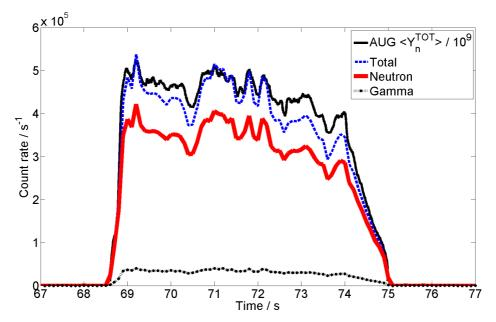
Fig. 10: (Color online) Comparison of count rates measured by the CNS with respect to the 100 ms time averaged AUG neutron yield  $\langle Y_n^{TOT} \rangle$  (divided by 10<sup>9</sup>) during AUG discharge 24151.
