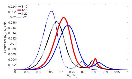
Fig. 7: (Color online) Examples of normalized  $Q_S/Q_L$  distributions relative to different S-L gate combinations. The peak on the left hand side corresponds to neutron events while the one on the right to  $\gamma$ 's. The maximum FOM value of 1.38 corresponds to S = 4 samples and L = 15 samples.
