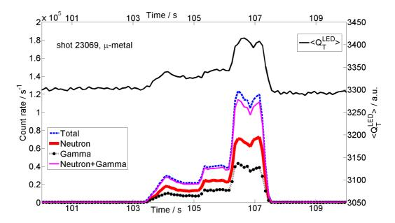
Fig. 4: (Color online) Same as in Fig. 3 but for AUG discharge 23069. The average LED pulse area  $\langle Q_T^{LED} \rangle$  follows exactly the count rate variation since the magnetic effects on the PMT are suppressed by the external  $\mu$ -metal shielding.
