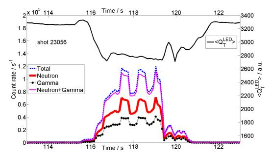
Fig. 3: (Color online) Count rates as a function of the DPSD acquisition time for the total, neutron and  $\gamma$  events measured by the CNS in AUG discharge 23056. On the top, the evolution of the average LED pulse area  $\langle Q_T^{LED} \rangle$  during the discharge is shown.
