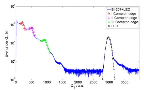
Fig. 1: (Color online) The <sup>207</sup>Bi PHS (the distribution of the events as a function of their pulse height  $Q_T$ ) measured with CNS. The Compton edges of the <sup>207</sup>Bi  $\gamma$ -rays and the LED peak have been fitted for assessing the performance of the BC501A liquid scintillating detector of the CNS.
