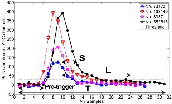
Fig. 5: (Color online) Examples of pulse shapes recorded in discharge 24151 with their corresponding number as recorded in the data set. Information is given on the DPSD acquisition trigger threshold at 10 mV. For pulse 583818, the regions of interests for n- $\gamma$  discrimination, namely, pre-trigger and gates S, L and T (i.e., the pulse length) are shown.
