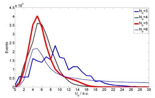
Fig. 6: Frequency distributions of the uncertainties  $U_o$  associated to the offset value calculated considering a number of pre-trigger samples  $N_o = [3, 6]$ .  $N_o^* = 5$  samples is the optimal number of samples for the offset reduction of the data because of its lowest average uncertainty value of 5 a.u..
