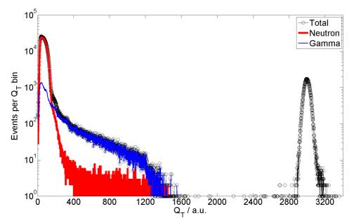
Fig. 9: (Color online) PHS  $Q_T$  of total, neutron,  $\gamma$  and LED events. The LED events are peaked about the reference LED pulse area  $Q_T^{\text{LED}*} = 3000$  a.u. after the PHS has been corrected.
