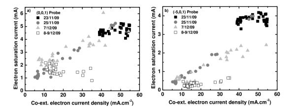
**Figure 4.** a) and b) show the variation of the electron saturation current with the co-extracted electron current density for the (0,0,1) and (-5,0,1) probes respectively.
