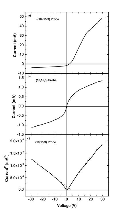
**Figure 6.** a) present a Langmuir probe characteristic recorded by the (-10,-15,3) probe, b) is the (10,15,3) probe characteristic, while c) is the  $i^2$  against V plot of the b figure.
