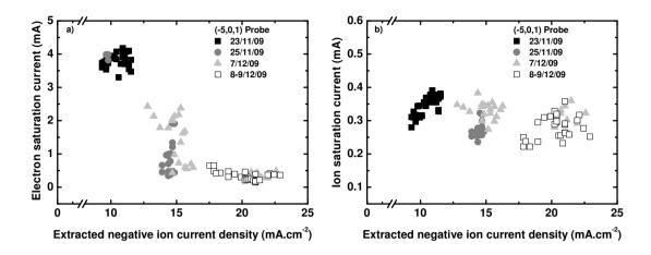
**Figure 5.** a) and b) present the evolution of the electron and ion saturation current of the probe as a function of the extracted negative ion current density.
