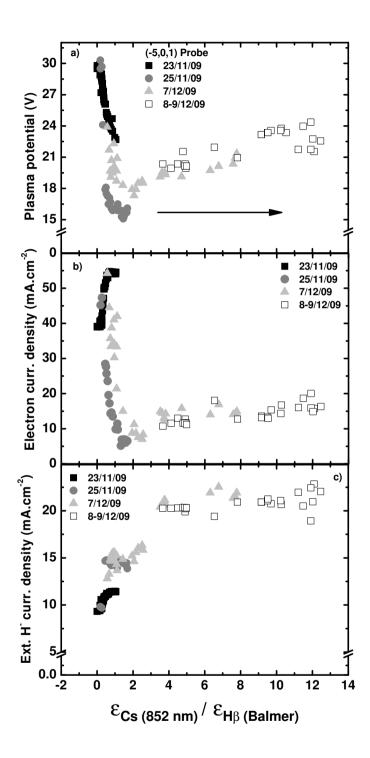
**Figure 3.** a) represents the plasma potential variation, b) the co-extracted electron current density and c) the extracted negative ion current density over days versus the spectroscopy emissivity line ratio. The arrow indicates the evolution over days
