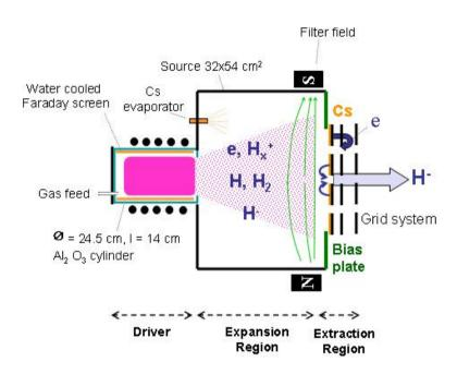
Figure 1. Schematic representation of the IPP RF source.
