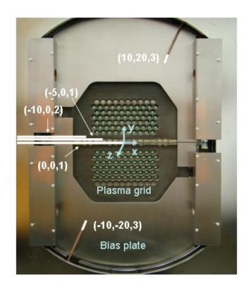
**Figure 2.** Picture of the PG. The location of the five pin probes is indexed by their position (in centimeters), the associated direct referential is in orange.
