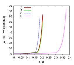
The right figure compares the results for the reference case (A) – parameters as given above – with those for doubled temperature (B), doubled density (C) and doubled conductivity of the first wall (D).
