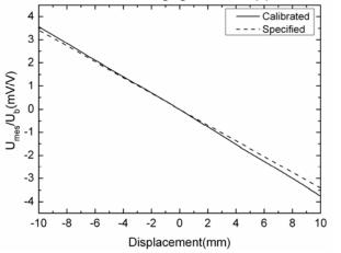
Fig. 7. Bridge voltage divided by power vs. displacement at RT.
