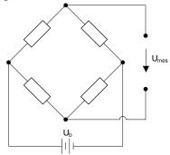
Fig. 3. Wheatstone full bridge circuit.
