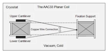
Fig. 9. The installation of the cantilever system on the planar coil AAC33.
