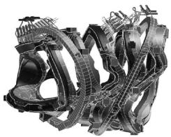
Fig. 1. Half module of the W7-X superconducting coil system.
