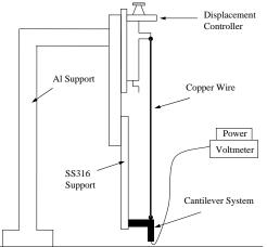
Fig. 6. Experimental setup for RT measurements.
