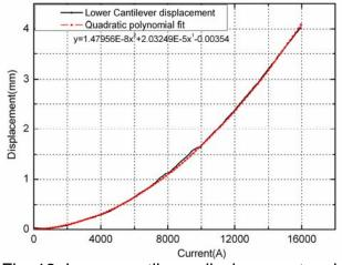
Fig. 12. Lower cantilever displacement variation during the first excitation.
