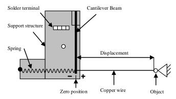
Fig. 4. The schematic of the displacement measurement system.
