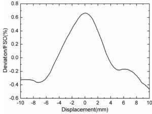
Fig. 8. Deviation divided by FSO vs. displacement at RT.
