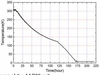
Fig. 10. Cool down process of the AAC33 coil.
