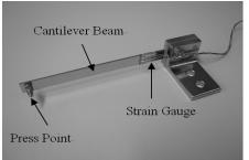
Fig. 2. The commercial strain type displacement transducer.
