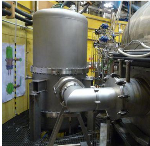
Fig. 2. Test cryostat attached to the large TOSKA cryostat with transfer line needed for helium feeding. The current supply to feed the current leads is connected from below.
