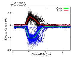
**Figure 2:** ELM averaged divertor currents. The currents are measured as flowing into a divertor tile.
