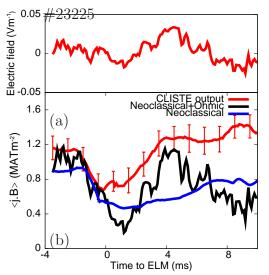
Figure 4: (a) shows the electric field calculated at the peak bootstrap position using a resistive current propagation model. (b) shows the flux surface averaged current density from CLISTE (red),  $\langle j_{neo} \cdot B \rangle$  (blue) and  $\langle j_{neo} \cdot B \rangle + \langle j_{Ohmic} \cdot B \rangle$  (black). will also be analysed in order to evaluate differences between slow and fast ELM cycles.
