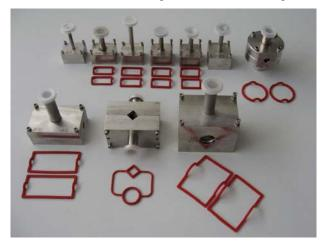
Fig.2 Set of solid test chambers for leak testing of weld seams
