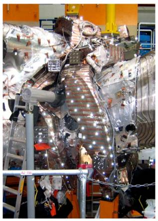
Fig.3 Photogrammetry of an adjusted coil
