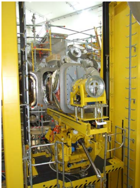
Fig.10 Large thermal insulated port fixed on the ramp. The ramp operates from a platform on the outer tower.
