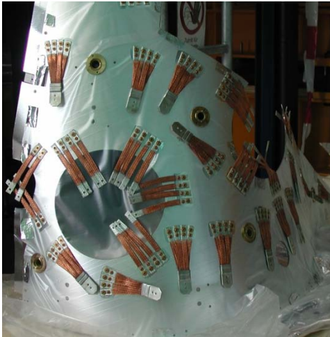
Fig.6 Copper braids on the plasma vessel shield
