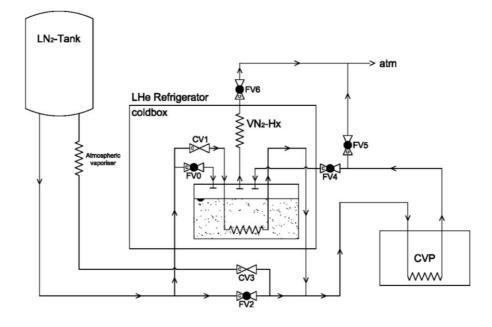
Fig.4 2-phase LN2 cooling scheme of CVP.
