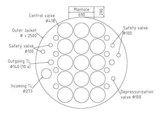
Fig.5 Top view of CVP valve box
