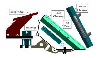
Fig.2 Main components of a CVP
