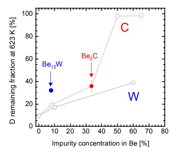
**Figure 4**: D remaining fraction at 623 K in Be-containing samples as a function of each impurity (W or C) concentration in Be.
