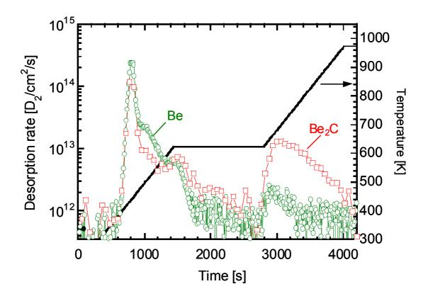
**Figure 2**: Thermal desorption spectra of D from Be and Be<sub>2</sub>C samples under the temperature programmed heating with 20 min. hold at 623 K (350 C). D implantation to those samples was done at room temperature.
