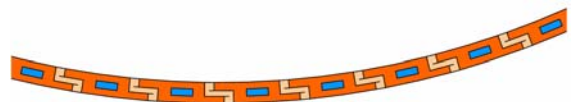
Fig. 2. Cross section of the Faraday shield with z-shaped slits and water cooling channels
