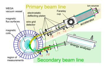
Fig. 1. (colour online) Scheme of the HIBP installed at the WEGA stellarator.
