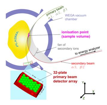
Fig. 2. (colour online) HIBP arrangement with the additional primary beam detector array. The plasma shape is shown for  $I_{tor}$ =3366 A in the toroidal coils and  $I_{hel}$ =4711 A in the helical coils respectively.  $\alpha$ 1,  $\alpha$ 2, and  $\beta$ 1 plates define the insertion position and the angle of primary beam,  $\alpha$ 3 and  $\beta$ 2 plates control the sample volume position along the primary beam.
