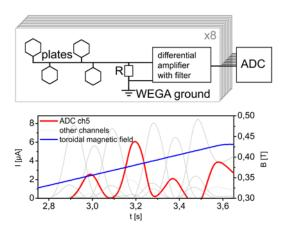
Fig. 3. (colour online) Simplified scheme of the array plates connection and typical signals obtained during a magnetic field scan.
