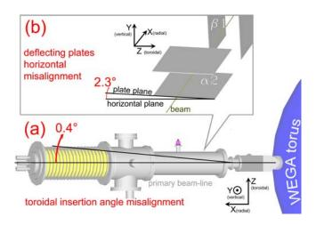
Fig. 5. (colour online) Geometrical misalignment of the primary beam line toroidal angle (a) and deflecting plates horizontal position (b)
