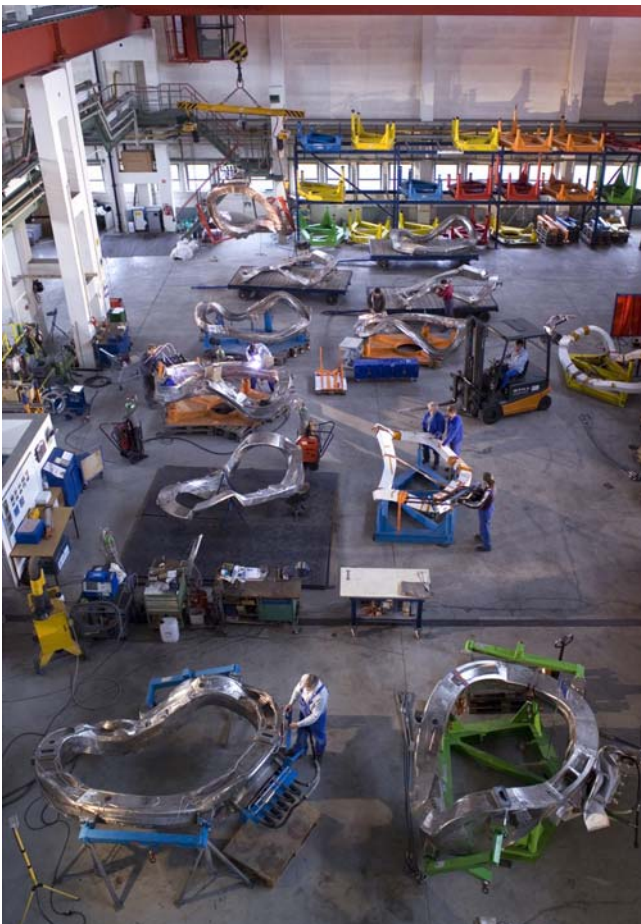
Figure 2: Non-planar coil assembly at BNG site in Zeitz.
