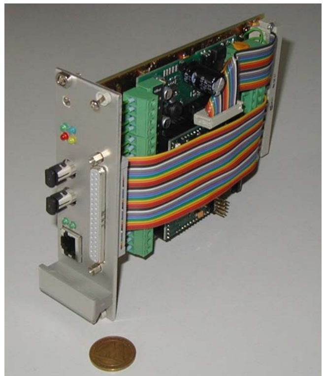
Figure 23: The gyrotron controller with Ethernet, optical fiber and Sub-D connectors.
