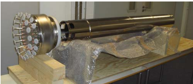
Figure 26: Vacuum interface flange for the B-port and the guiding tube for the ECRH transmission measurement waveguides.
