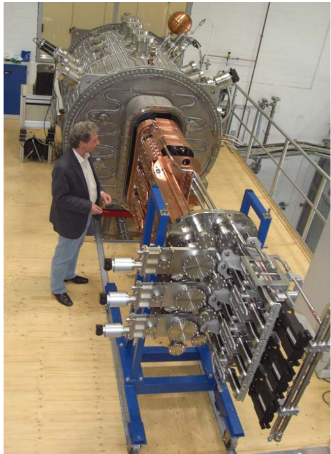
Figure 25: ECRH launcher before insertion in the MISTRAL chamber for vacuum leak check and mechanical cyclic fatigue tests under vacuum.
