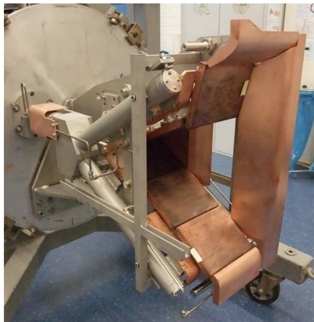
Figure 30: Ion dump capable to absorb the unneutralized power from one beam of a neutral beam injector.
