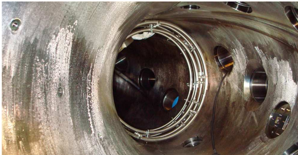
Figure 4.13: Magnetic diagnostics mounted inside the vacuum vessel where the access is only possible through the existing ports. The picture was also made through one port.
