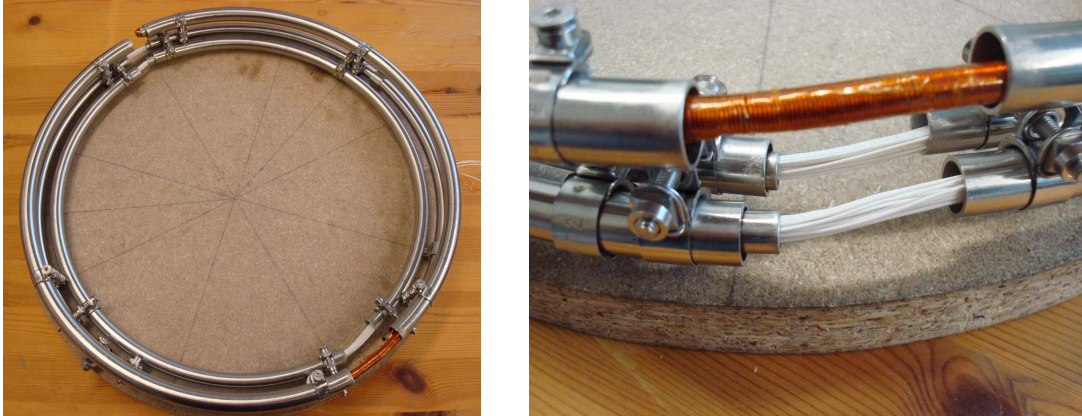
(a) Open state of the system to enable flipping of both bows ensuring the lead through in vacuum vessel (b) Zoomed figure showing cable route in the shielding pipes
