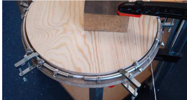
Figure 4.4: Mounting device for diamagnetic loop
