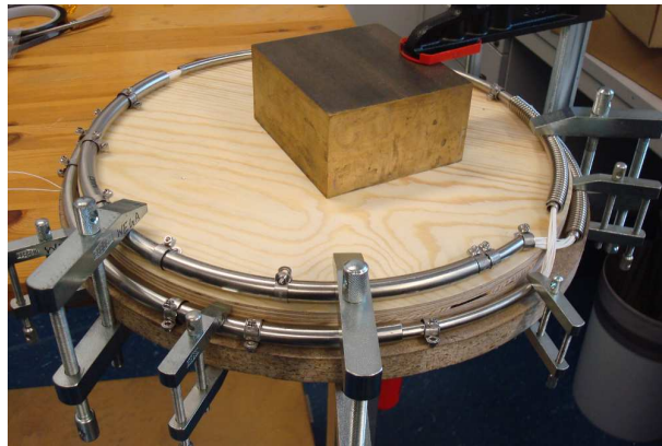
Figure 4.6: Mounting structure for assembling the compensation coil
