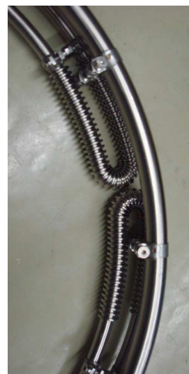
(b) Bent corrugated tubes to realize the cable path of the compensation coil
