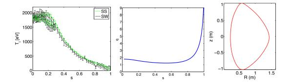
Figure 1: The ion temperature profile, q-profile and the plasma shape of the MAST discharge #22807 at 0.25s. The two measurements of ion temperature refer to the two independent neutral beams used by the CXRS system. The inboard side measurements are folded onto the outboard side in s < 0.3. The internal transport barrier (ITB) with steep  $\nabla T_i$  is in the region 0.3 < s < 0.5.
