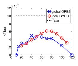
Figure 2: The linear growth rates of ITG modes in MAST discharge #22807 with a local GYRO (red) and a global ORB5 (blue) simulation without flow shear.
