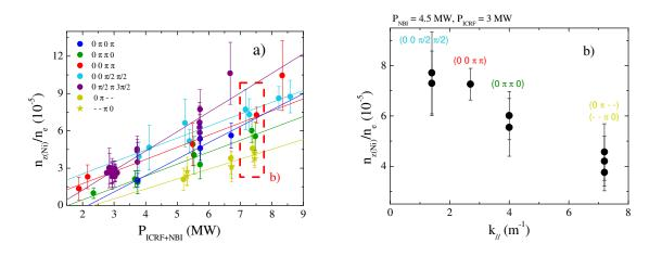
Figure 1. a) Correlation between Ni concentration ( $r/a \approx 0.5-0.6$ ) and total applied heating power for different A2 antenna phasings, and b) Nickel concentration vs parallel wave number  $k_{ll}$  for selected points in a) with 3 MW of ICRF power and 4.5 MW of NBI.
