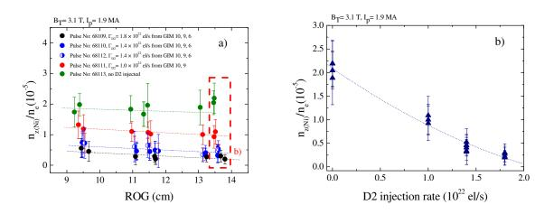
Figure 2. a) Correlation between Ni concentration ( $r/a \approx 0.5-0.6$ ) and antenna–separatrix distance ROG, and b) Ni concentration ( $r/a \approx 0.5-0.6$ ) vs different levels of injected D2 gas for selected points in a) with ROG around 14 cm (ITER-AT configuration).
