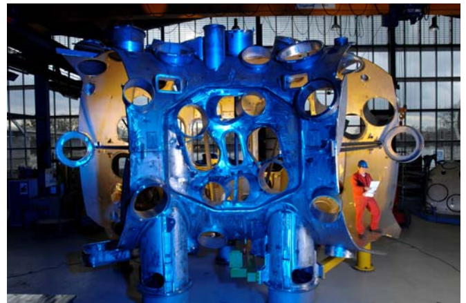
Figure 3. One module of the Outer Vessel during a test assembly
