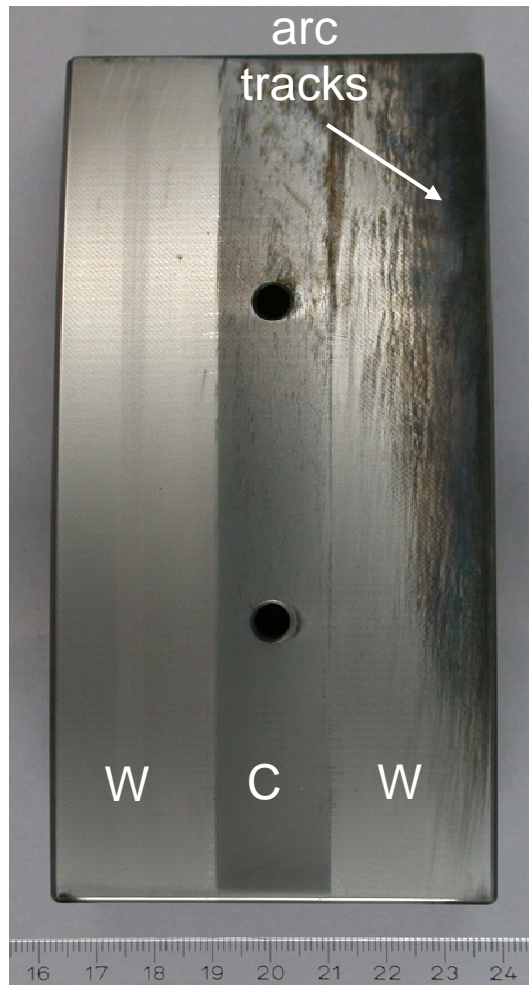
Fig. 2: Marker stripes on inner divertor tile 5 after exposure during the 2007 campaign. The markers consisted of a 300 nm thick W marker coating and an uncoated carbon area in the middle of the tile. The left hand side of the tile was plasma-shadowed, the right hand side was plasma-exposed. A large number of arc tracks was observed after exposure.
