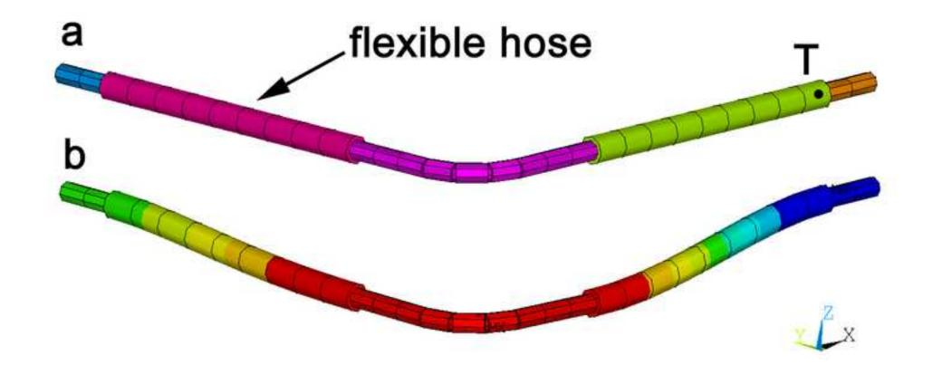
Deformation of cryo-pipe system Click here to download high resolution image
