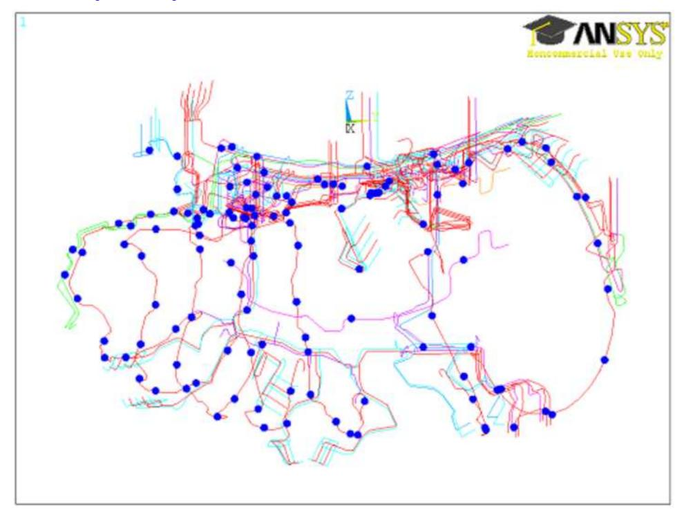
Typical pipe supports mounted on coil Click here to download high resolution image
