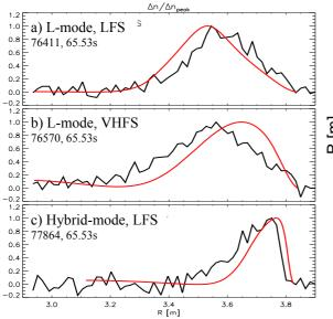
Fig 2: Normalised particle deposition (black) compared with ablation predictions (red, NGPS model without drift).
