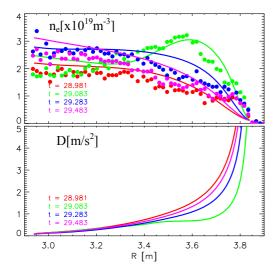
Fig 4: Fully predictive JETTO simulation of density profile evolution in the vicinity of a LFS pellet injected into Ohmic plasma (#76570). Top: density profiles (lines: JETTO. points: HRTS.). Bottom: particle diffusivities
