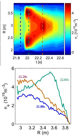
Fig 3: Density profile evolution (#77421). Top: contour plot. Bottom: HRTS profiles before, immediately after injection and after particle diffusion (times of vertical lines in the top box)
