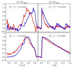
Fig 1: Normalised particle deposition (left) and density decay (right). Top row: H-mode. Bottom row: L-mode. Blue: LFS. Red: VHFS.
