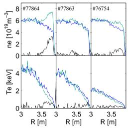
Fig. 5 Electron density and temperature after the pellet injection in three discharges #77864 (VHFS  $P_{NBI} = 21$  MW, t = 7.4 s) #77863 (LFS  $P_{NBI} = 21$  MW, t = 6 s), #76754 (LFS  $P_{NBI} = 6$  MW t = 9.3 s). The blue line is before pellet injection, the green line is after pellet injection. The black line is the difference.
