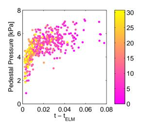
Fig. 3 Electron pressure at the top of the pedestal as function of the delay from the previous ELM. The color scale is related to the amount of injected deuterium.
