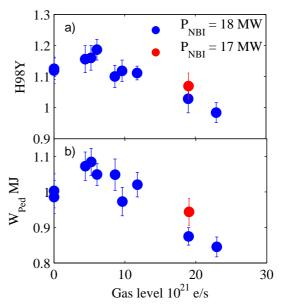
Fig. 2 Normalized confinement and pedestal energy content as function of the gas injection rate for the hybrid discharges. The pedestal energy content is calculated assuming that the ion contribution is equal to the electron one.
