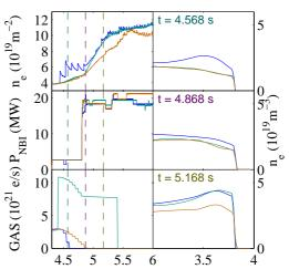
Fig. 6 density during the prelude phase for the shots: #77868 (blue), #77869 (green), and #77867 (red). Pellets were injected in shot #77868, while #77869 was fuelled with gas puffing
