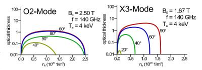
Figure 1: Angular dependence of the optical thicknesses of the O2- and X3-mode. [2, 3]
