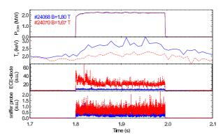
Figure 3: Discharges with X3-heating and B= 1.67 T (red, dashed) and 1.8 T (blue). From top to bottom: ECRH power, electron temperature, ECE-diode and sniffer probe.
