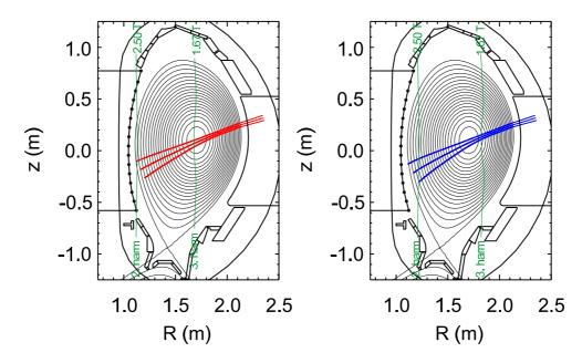
Figure 2: TORBEAM calculations for the X3-heating scenario at a magnetic field of 1.67 T (left, red) and 1.8 T (right, blue).
