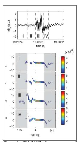
Figure 1. JPN 76697. Spontaneous type-I ELM. Top: magnetic perturbations. Bottom: spectrum P(n,f) during phases I-IV. Shaded areas are affected by large uncertainties.
