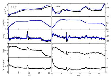
Fig. 1. Comparison between experimental readings (black) and state space model outputs (blue). In top-down order are shown the plasma internal inductance, plasma current, voltage  $V_C$ , boundary voltage  $V_B$  and plasma resistance R.
