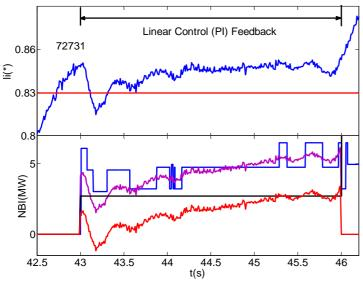
experiments with NBI have shown the feasibility of feedback to control the inductance. Fig 4 shows the results of a feedback experiment during the ramp-up phase. The natural tendency of li to increase with time in ohmic shots is compensated by NBI heating reducing the plasma resistance, and then lowering the inductance. This control test was performed with a linear PI control without with Kp=80, Ki = 0.5, during the ramp-up phase, without compensation of non linearities,
