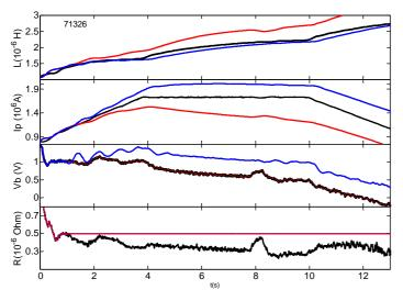
Fig.2 Simulation of inductance tracking. Reference discharge is shown in black. Red traces correspond with an open loop simulation with identical boundary voltage to the reference discharge. Blue traces are feedback simulations. In both red and blue cases Ip and L are obtained from the state space model subject to the same constant plasma resistance shown. In the red case the boundary voltage matches the reference discharge, while in the blue case the boundary voltage is issued by the control.
