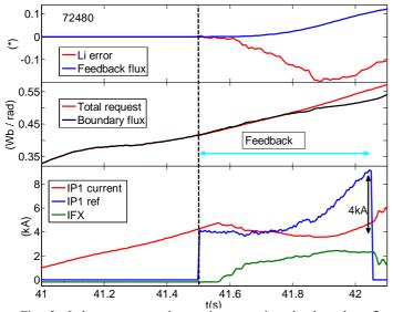
Fig. 3. Inductance control experiments using the boundary flux control tool as actuator. From top down are shown the Internal inductance error signal, flux request and relevant PF currents.
