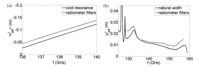
Figure 3: Localisation and spatial resolution for standard ECE diagnostics (radiometer filters) for realistic conditions at W7-X. (a) Emission layer position  $< r_{eff}^i >$ . In the plasma center, the distance from  $< r_{eff}^i >$  (dashed) to the cold resonance (solid) is about 2 cm. (b) Emission layer width  $\Delta r_{eff}^i$  (dashed). In comparison the emission layer width for individual frequencies (solid) is given.
