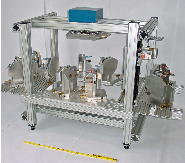
Figure 2: Set up of the quasi-optical diplexer consisting of the ring resonator (top and - non-visible - bottom mirror and left and - non-visible - right grating mirror, as well as 4 two-mirror matching optics for incoming and outgoing beams.
