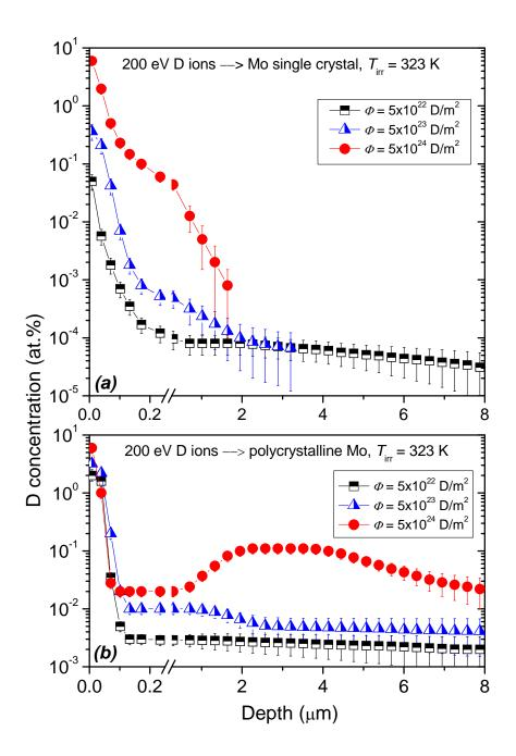
Figure 1. Depth profiles of deuterium trapped in (a) single crystal Mo and (b) polycrystalline Mo, both irradiated with 200 eV D ions at  $T_{irr} = 323$  K to various fluences.
