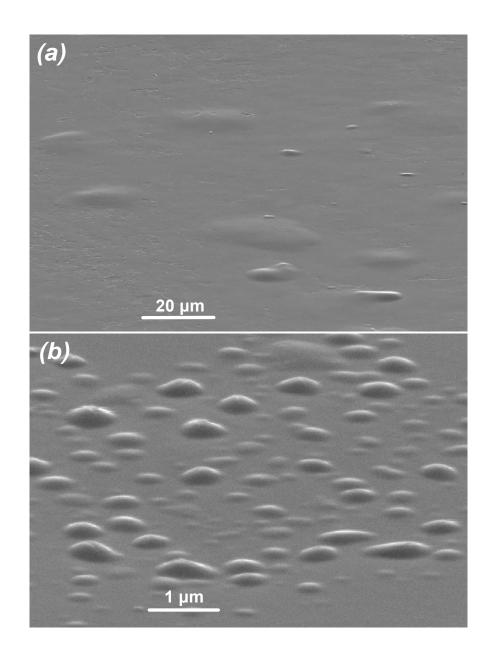
Figure 2. Blisters formed during irradiation with 200 eV D ions at  $T_{\rm irr} = 323$  K: (a) polycrystalline Mo with fluence of  $5\times10^{24}$  D/m<sup>2</sup>, and (b) MoO<sub>3</sub>/polycrystalline Mo sandwich with fluence of  $5\times10^{22}$  D/m<sup>2</sup>. The surfaces were analysed by a SEM at a tilt angle of 70 degrees.
