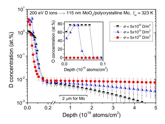
Figure 3. Depth profiles of deuterium trapped in 115 nm  $MoO_3$ /polycrystalline Mo sandwich irradiated with 200 eV D ions at  $T_{irr} = 323$  K. Variation of the oxide film thickness due to the D ion irradiation is shown in the insert.
