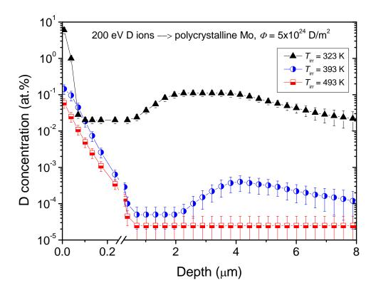
Figure 4. Depth profiles of deuterium trapped in polycrystalline Mo irradiated with 200 eV D ions at various temperatures to a fluence of  $5 \times 10^{24}$  D/m<sup>2</sup>.
