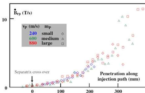
Figure 3: Pellet induced magnetic perturbation versus pellet position along the injection path, separatrix position defines 0. At the given plasma position, the same magnitude for the pellet driven magnetic response is observed for any pellet speed and/or mass applied (inserted legend show different pellet velocities and sizes used during the study).
