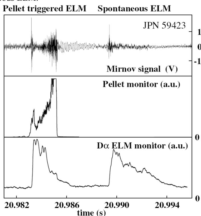
First results of spectral analysis of magnetic perturbations, based on wavelets, indicate that ELM triggered by pellets can be described as explosive instabilities, with a growth dynamics comparable to that of their spontaneous counterparts.
