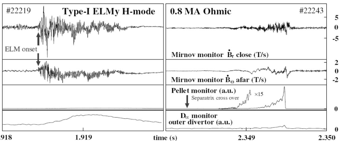
Figure 2: MHD perturbation during spontaneous type-I ELM and pellet injection into OH plasma (identical scales). This pellet driven magnetic perturbation in OH represents the weakest observed impact of all available pellet parameters; it exceeds the magnitude of the MHD activity observed at the very onset of the ELM (indicated by the arrows).
