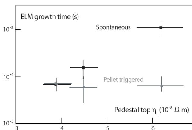
Figure 1: When creating a cooler edge at higher density, e.g. the pedestal top resistivity (parallel Spitzer) increases as the plasma undergoes a transition from type-I to type-III ELM regime. While the spontaneous ELM growth times rise significantly (note logarithmic scale), triggering maintains a fast ELM onset. Data from hot edge type-I, Ar seed cooled type-I and type-III ensembles (left to right); all discharges at  $I_p = 1$  MA.
