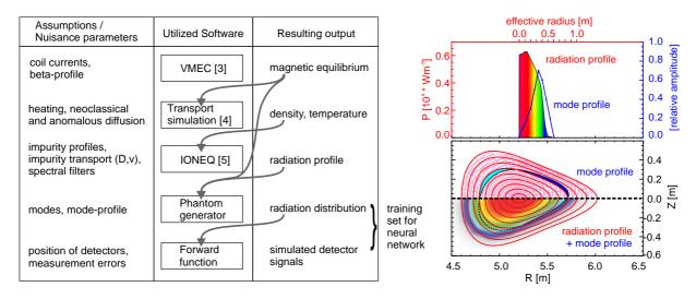
Figure 1: Left: Simulation software chain used to create the inputs and outputs for training the NNs. Dependencies and nuisance parameters are also listed. Right: m=2 mode perturbs the magnetic flux-surfaces (VMEC output). The radiation profile (from IONEQ) is mapped onto these perturbed flux-surfaces.
