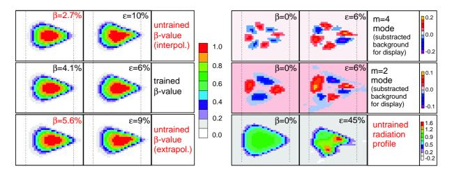
Figure 2: Left: comparison between phantom and reconstruction data for selected phantoms with different  $\beta$ -values. Right: comparison of mode reconstruction and a failing reconstruction for a phantom with a different (untrained) radiation profile.
