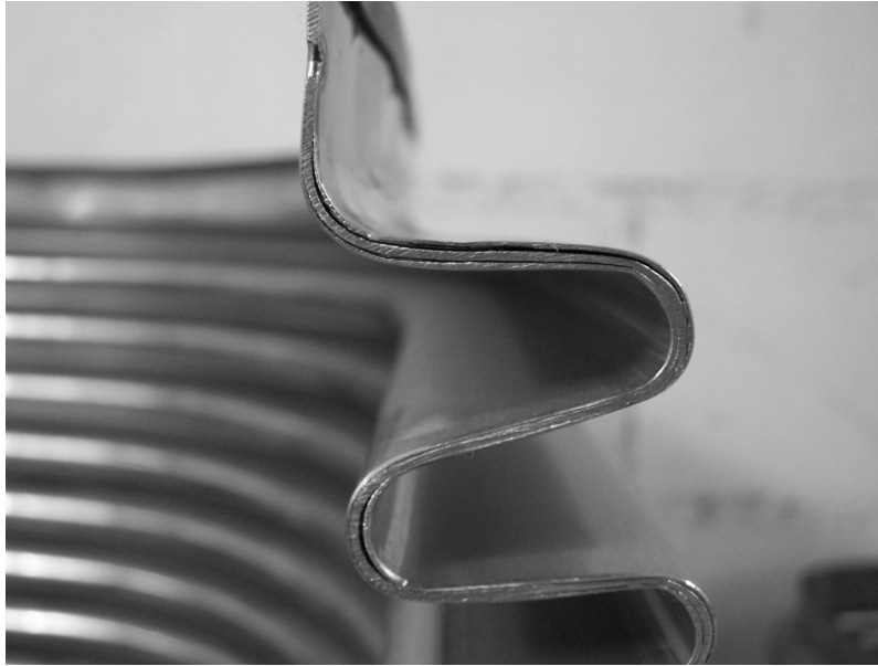
Fig. 1. Cut of three layers, rectangular bellows
