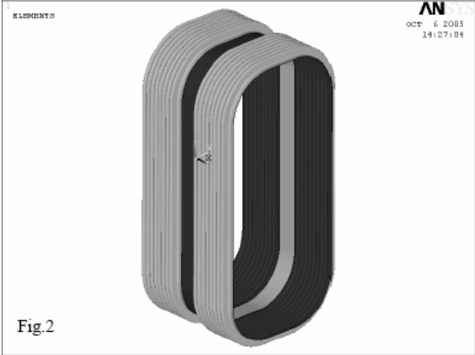
Fig. 2. Rectangular bellows modelled in FEM ANSYS
