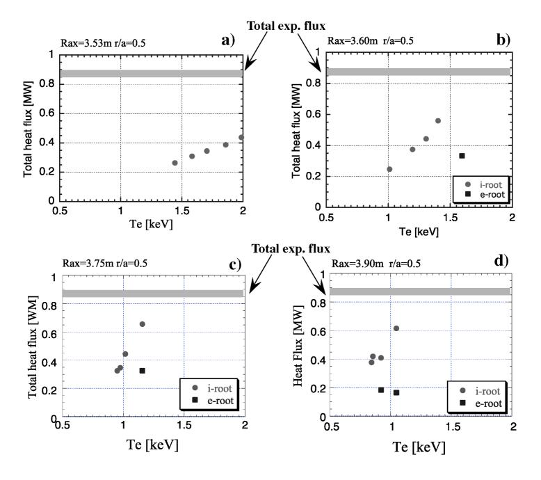
Fig. 8 Plots of the total heat flux of neoclassical transport evaluated by DCOM at r/a = 0.5 as a function of the electron temperature for four LHD configurations; a)  $R_{ax}=3.53$ m, b)  $R_{ax}=3.60$ m, c)  $R_{ax}=3.75$ m, d)  $R_{ax}=3.90$ m.
