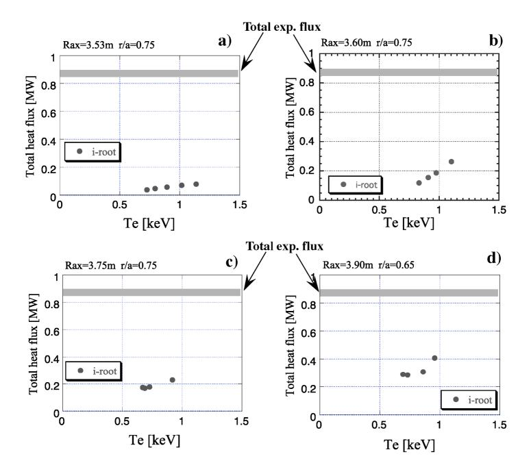
Fig. 9 Plots of the total heat flux of neoclassical transport evaluated by DCOM at r/a =0.75 (0.65 for the  $R_{ax}$ =3.90m configuration) as a function of the electron temperature for four LHD configurations; a)  $R_{ax}$ =3.53m, b)  $R_{ax}$ =3.60m, c)  $R_{ax}$ =3.75m, d)  $R_{ax}$ =3.90m
