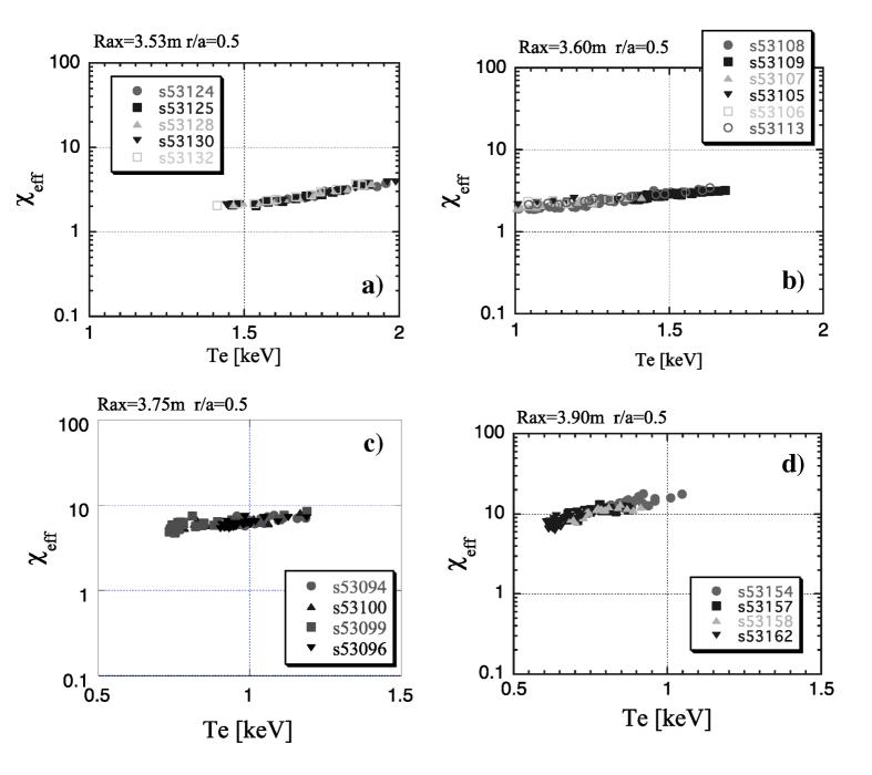
Fig. 5 Plots of the effective heat transport coefficient at r/a =0.5 as a function of the electron temperature for four LHD configurations; a)  $R_{ax}$ =3.53m, b)  $R_{ax}$ =3.60m, c)  $R_{ax}$ =3.75m, d)  $R_{ax}$ =3.90m.
