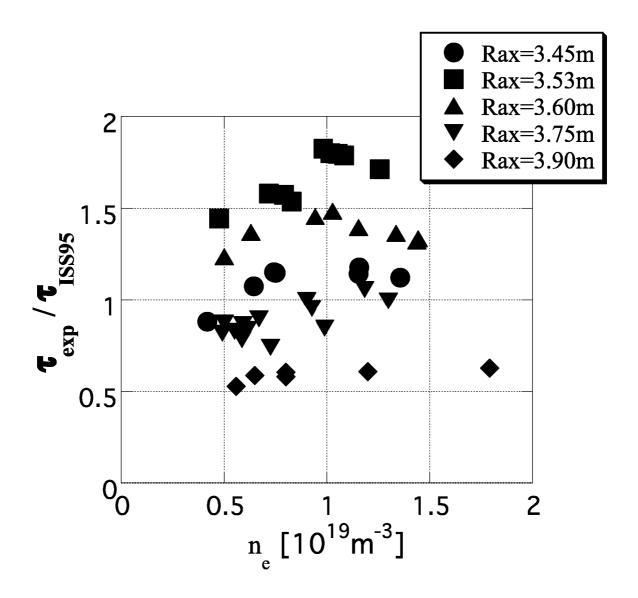
Fig. 3 Enhancement factor of the global energy confinement time relative to the ISS95 scaling law as a function of the line averaged density for five configurations of LHD.
