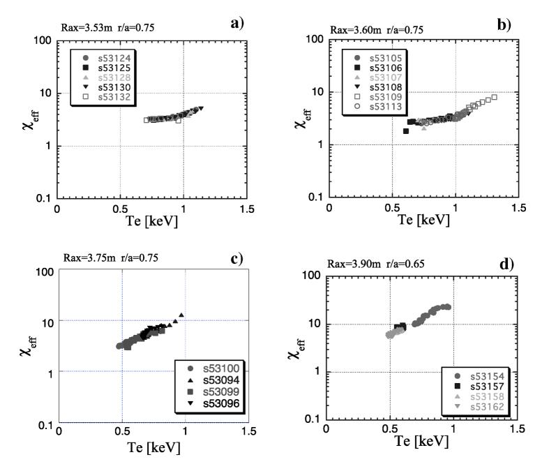
Fig. 7 Plots of the effective heat transport coefficient at r/a =0.75 (0.65 for the R<sub>ax</sub>=3.90m configuration) as a function of the electron temperature for four LHD configurations;
