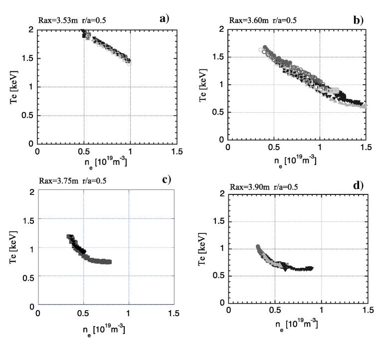
Fig. 4 Plots of the electron temperature at r/a =0.5 as a function of the line averaged density for four LHD configurations; a)  $R_{ax}$ =3.53m, b)  $R_{ax}$ =3.60m, c)  $R_{ax}$ =3.75m, d)  $R_{ax}$ =3.90m.
