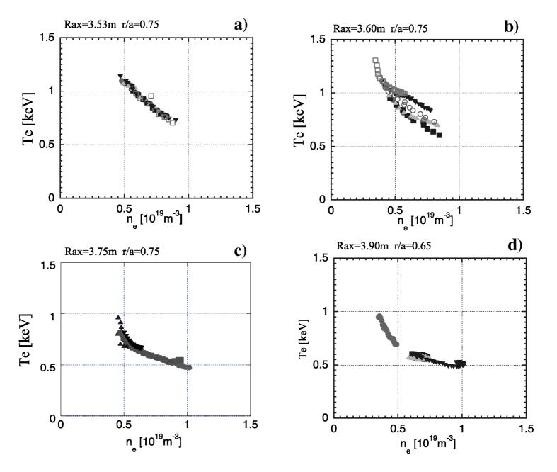
Fig. 6 Plots of the electron temperature at r/a =0.75 (0.65 for the  $R_{ax}$ =3.90m configuration) as a function of the line averaged density for four LHD configurations; a)  $R_{ax}$ =3.53m, b)  $R_{ax}$ =3.60m, c)  $R_{ax}$ =3.75m, d)  $R_{ax}$ =3.90m.
