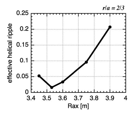
Fig. 1 Effective helical ripple at r/a=2/3 as a function of magnetic axis position in major radius in LHD evaluated by DCOM.
