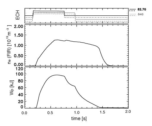
Fig. 2 Typical time development of the ECH plasma discharge in LHD (Rax=3.65m); ECH heating power (top), line averaged density (center) and stored energy (bottom).
