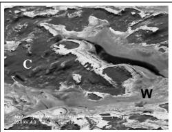
**Figure 4** SEM picture from the area of heaviest erosion on outer tile 7.
