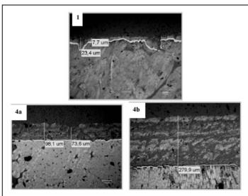
Figure 2 Metallographic cross-sections from samples of inner divertor vertical tile 1 and base tile 4 (4a on horizontal part and 4b on inclined part of tile 4).
