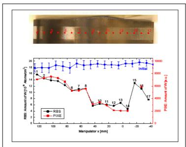
Figure 3 RBS and PIXE profile of the tungsten areal density along outer vertical tile 7.
