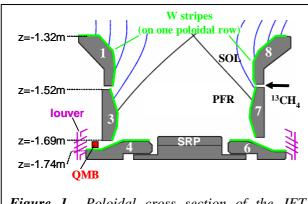
Figure 1 Poloidal cross section of the JET MkIIGB-SRP divertor.
