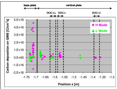
Figure 6 Carbon deposition on the QMB in dependence on strike point position during MkIIGB-SRP campaigns.
