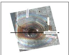
Figure 7 Photograph of front side of the inner heat shield of the QMB.
