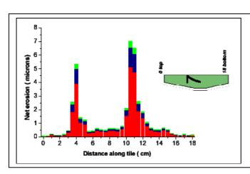
Figure 5 Calculated net tungsten erosion along tile 7 after campaigns C5–C14. Red bars: erosion due to background carbon; Blue bars: erosion due to recycled physically sputtered carbon; green bars: erosion due to recycled chemically eroded carbon.
