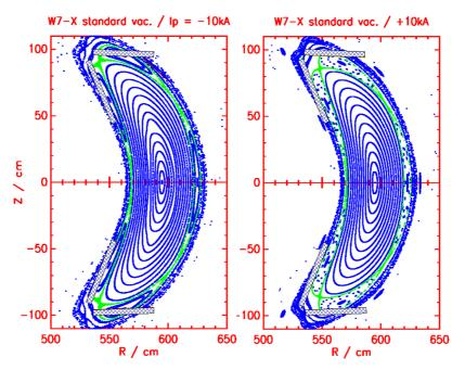
FIG. 1: W7-X standard magnetic configuration for different bootstrap current values (+/-10 kA). The green point indicate the separatrix. The X point distance to the target plates (shaded area) varies like 2.5mm / kA.
