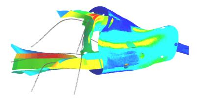
FIG. 2: Heat loads on the W7-X plasma vessel and divertor structure by plasma radiation emitted from the X-Points (scattered gray line). The color indicates the heat-flux, red 130 kWm<sup>-2</sup> down to blue 0 kWm<sup>-2</sup>.
