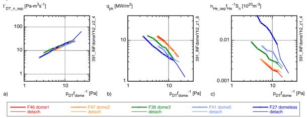
Fig. 2. Neutral DT influx to the core (a), peak power loading of the target (b), and helium density at the separatrix (c) vs. the normalised neutral pressure in the PFR for different dome configurations. The helium density is scaled with the fusion power and pumping speed, see [6, 3] for details. f<sub>dome</sub> is 1 (F46), 0.84 (F47), 0.74 (F38), 0.68 (F41) and 0.69 (F27).
