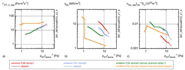
Fig. 4. Neutral DT influx to the core (a), peak power loading of the target (b), and helium density at the separatrix (c) vs. the normalised pressure in the PFR for the different locations of the separatrix strike-points. The data for the standard configuration are also shown for comparison.  $f_{dome}$  is 1 (F46), 0.68 (F41) and 0.75 (F42, F44). F42 is not in the same detachment state as the others. See also the caption for Fig. 2 for more detail.
