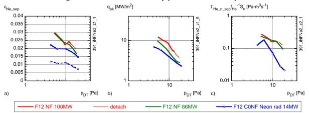
Fig. 5. Impurity concentration (solid: C, dashed: Ne) (a), peak power loading of the target (b), and helium atom flux across the separatrix (c) vs. the neutral pressure in the PFR without neon at 100 and 86 MW, and with 14 MW neon radiation at 100 MW input power to the SOL.
