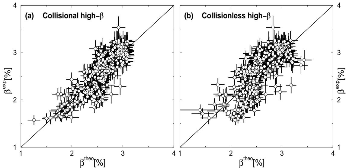
Figure 2: Experimental versus predicted plasma- $\beta$  for (a) the most probable model (collisional high- $\beta$ ) and (b) the second most probable model (collisionless high- $\beta$ ).
