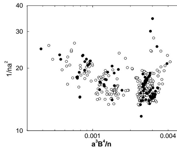
Figure 1: W7-AS high- $\beta$  data in the space of the Connor-Taylor variables:  $a^3 B^4 / n$  is assigned to a collisional model,  $1/na^2$  to high- $\beta$ . Open circles: full set of  $N=380$  data. Filled circles: subset of  $N=96$  data for  $0.45 < \tau < 0.49$ .
