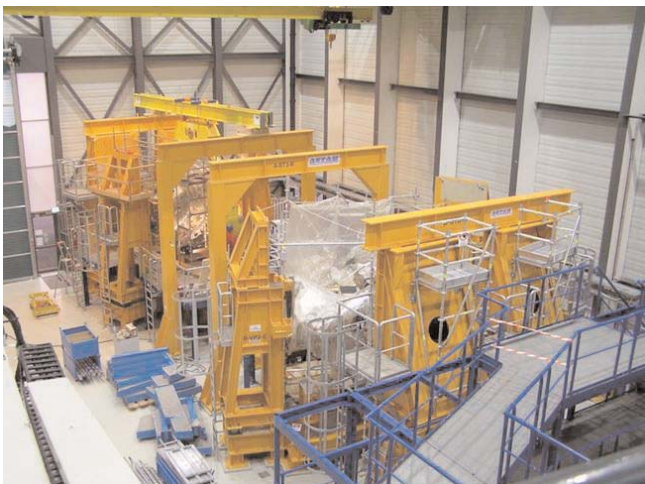
Figure 30: Two flip-symmetric half modules are being mounted in the pre-assembly hall
