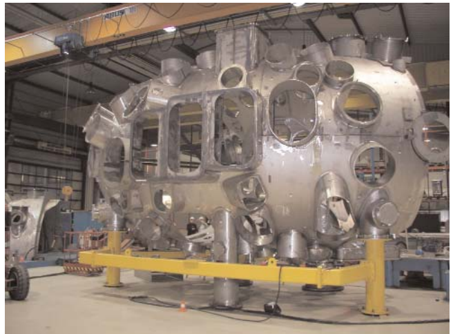
Figure 8: Pre-assembled lower and upper shells of module 5
