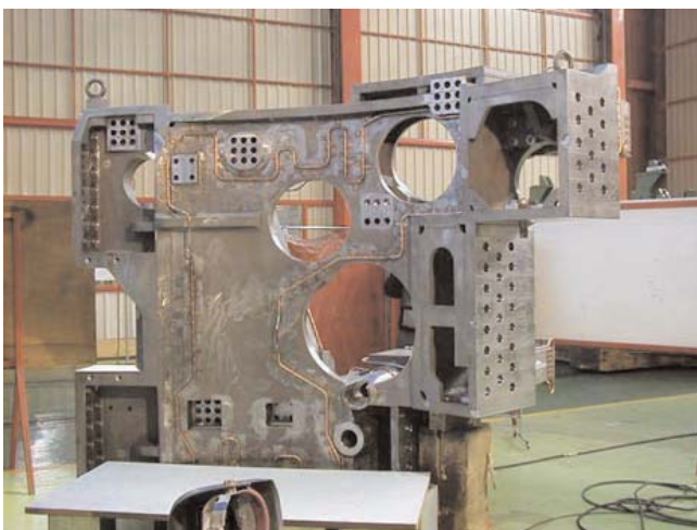
Figures 5 and 6: Installation of the cooling tubes and front view of module 5.0
