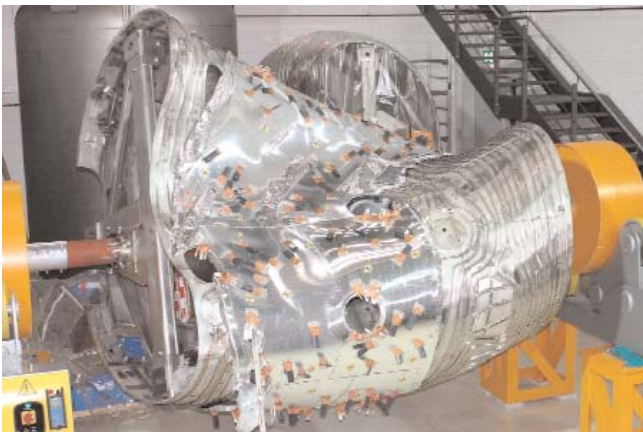
Figure 7: Mounting of the thermal insulation panel
