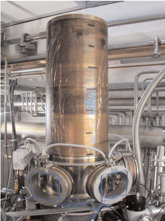
Figure 39: The TED Gyrotron with the transverse field sweeping coils
