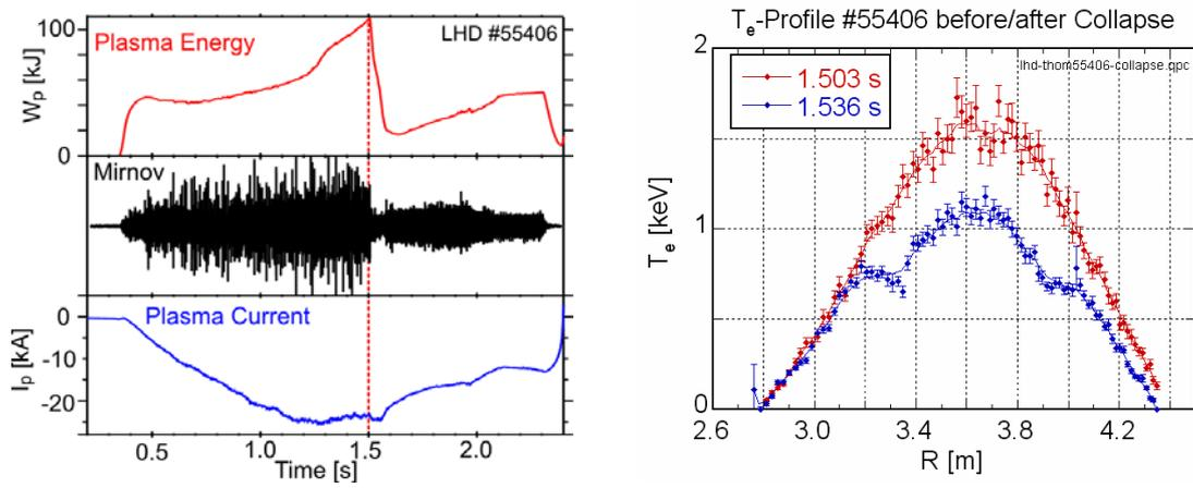
**Figure 11.** Collapse of plasma energy in LHD due to an  $m/n = 1/1$  interchange mode. A small  $\gamma$ -parameter ( $\gamma = 1.129$ ) along with co-current generates a low shear iota-profile with  $\iota = 1$  in the plasma core. A flattened region in the  $T_e$ -profile is formed during the collapse (right).
