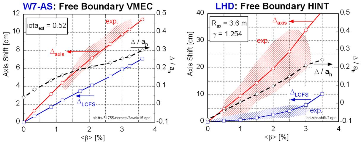
**Figure 6.** Free boundary VMEC (W7-AS, left) and HINT (LHD, right) predictions of  $\beta$ -induced horizontal shifts of the plasma axis (red), the LCFS (blue) and their difference (Shafranov shift normalized to horizontal plasma radius  $a_h$ , black dashed line, right scales). The shaded areas represent the range of available experimental data.
