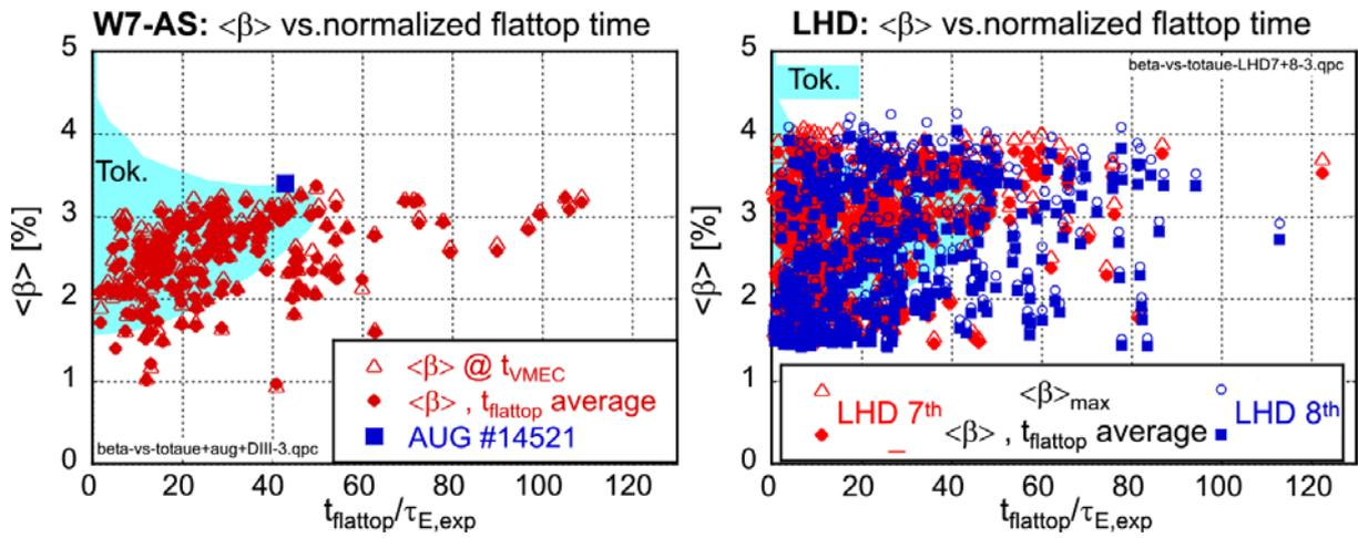
**Figure 2.** High- $\beta$  databases of W7-AS (left) and LHD (right, 7<sup>th</sup> & 8<sup>th</sup> campaign). Volume averaged  $\beta$  values are given as a function of the flattop time normalized to the confinement time. The open symbols refer to the time in the discharge, where the VMEC analysis was performed. The solid symbols represent time averages during the flattop. In addition, the typical range of tokamak data is indicated by the shaded area.
