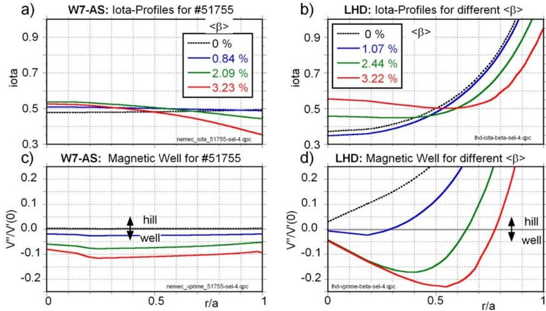
**Figure 1.** Finite- $\beta$  effects on radial profiles of the rotational transform  $\iota$  and the magnetic well depth  $V''(\rho)/V'(0)$  ( $V$ : volume,  $\rho = r/a$ ) calculated by the VMEC code for W7-AS (left) and LHD (right). The vacuum configurations are inward shifted ( $R_{ax} = 3.6$  m in LHD).
