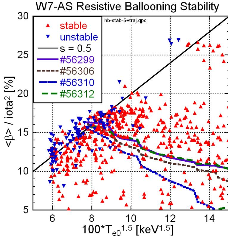
**Figure 12.** Database of  $\langle \beta \rangle$  normalized to  $\iota^2$  versus  $T_e^{3/2}$  of high- $\beta$  discharges in W7-AS. The parameters just prior to MHD collapses (solid triangles) are close to a critical value of the inverse linear growth rate (dotted line “ $s = 0.5$ ”). The solid lines are the trajectories of individual discharges until the collapse.
