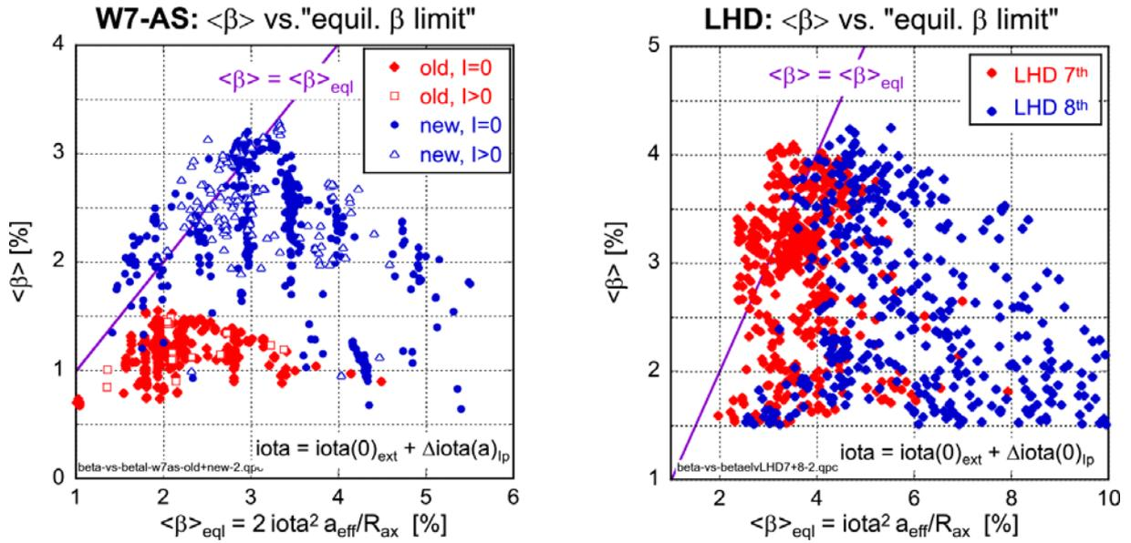
**Figure 5.** Achieved  $\langle\beta\rangle$  in W7-AS and LHD plotted versus  $c/A_p \tau^2 \equiv \langle\beta\rangle_{\text{eql}}$  as an estimate of an “equilibrium  $\beta$  limit” corresponding to  $\Delta/a = 1/2$  ( $c = 2$  for W7-AS,  $c = 1$  for LHD).
