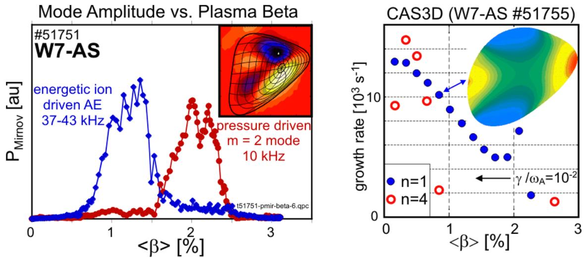
**Figure 9.** Mode amplitudes in W7-AS depending on  $\beta$ . The observed  $m/n = 2/1$  pressure driven mode (left, inset: X-ray tomogram) disappears above  $\langle\beta\rangle = 2.5\%$  in agreement with vanishing growth rates of global ideal modes as predicted by CAS3D (right).
