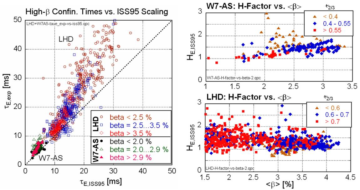
**Figure 3.** Comparison of experimental energy confinement times with the ISS95 scaling for same W7-AS and LHD high- $\beta$  databases as used in fig. 2 (left). The H-factors (enhancement  $\tau_{E,exp}/\tau_{E,ISS95}$ ) are given on the right.
