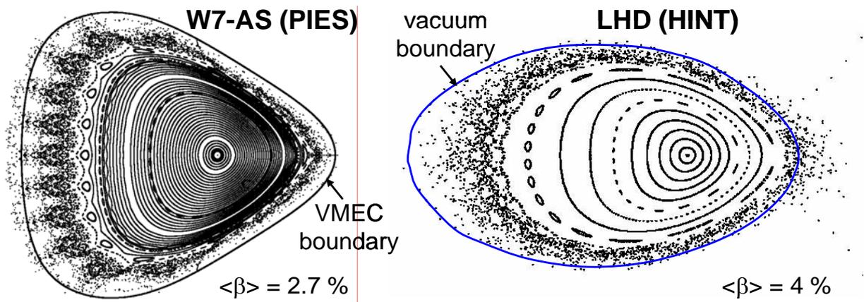
**Figure 7.** Free boundary high- $\beta$  equilibria as calculated for W7-AS with PIES (left) and for LHD with HINT (right). A large fraction of flux surfaces is predicted to be degraded by island formation and generation of stochastic field regions.
