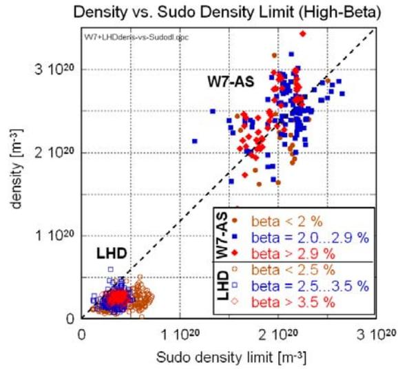
**Figure 4.** Densities for same W7-AS and LHD high- $\beta$  databases as used in fig. 2 (left) compared with Sudo density limit [28] (dashed line).
