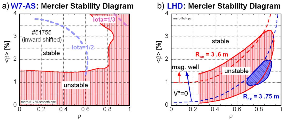
**Figure 8.** Mercier stability diagrams for W7-AS (left) and LHD (right) configurations. The W7-AS and LHD ( $R_{ax} = 3.6\text{ m}$ ) configurations are inward shifted and less stable.
