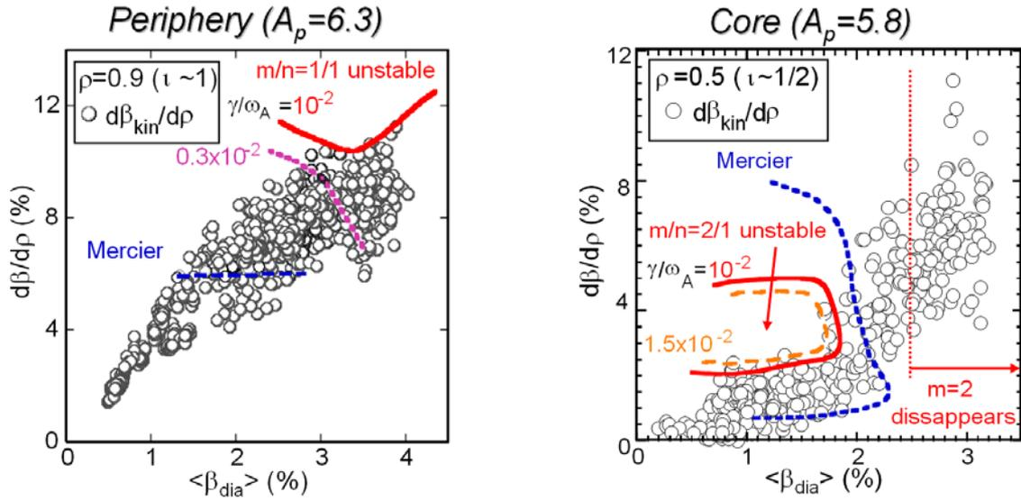
**Figure 10.** Observed gradients of  $\beta$  in LHD at the plasma periphery ( $\rho = 0.9$ , left) and in the core ( $\rho = 0.5$ , right) plotted against  $\langle\beta\rangle$ . Stability thresholds for the Mercier stability are significantly violated in experiment. The threshold for low- $n$  ideal interchange modes with growth rates  $\gamma/\omega_A = 10^{-2}$  is not exceeded in experiment. The presence of observed MHD modes correlates with the Mercier unstable region.
