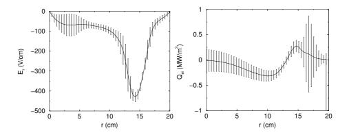
Figure 3: Radial electric field and electron-ion energy exchange term.
