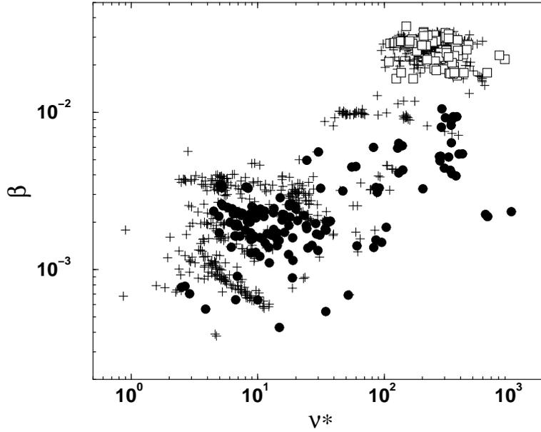
Figure 1: Examined W7-AS confinement data as a function of beta and collisionality (low-beta subset: circle, high-beta subset: squares, additional data in ISCDB: plus signs).
