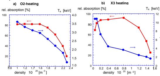
**Figure 2.** Single pass absorption for the O2-mode (left, squares)) and the X3-mode (right, squares)) as a function of density. The temperature (circles) was estimated according to the stellarator scaling for an input power of 10 MW.
