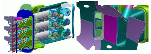
**Figure 3.** Right: ECRH plug-in launcher for the equatorial port in W7-X. Left: inside port design. Right: front view.
