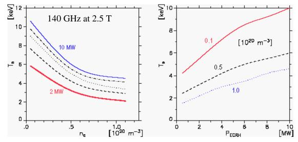
Figure 1, Expected central temperatures for X2-heating as a function of density and heating power.
