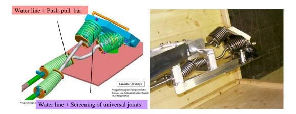
**Figure 4.** Tube spirals for a flexible cooling water supply of the front steering mirror. Left: CAD. Right: Mechanical realization in the ECRH mock-up launcher.
