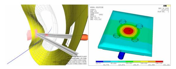
**Figure 5.** Left:Ray-tracing calculation for the optimum position of the O2 and X3 reflector tiles at the plasma vessel in-board side. Right: Heat load simulation of a strongly focused ECRH- beam (500 kW beam waste 20 mm) at the TZM-reflector tile.
