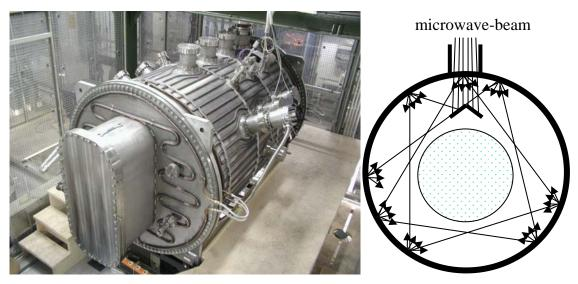
**Figure 6.** Left: ECRH stray radiation test chamber with a large W7-X equatorial port type A in front. Right: Scheme of stray radiation generation. The microwave beam is rotating in side the test in a whispering gallery mode. Every reflection at the rough in-vessel surface illuminates the shadowed central test volume.
