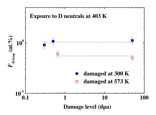
Fig. 3 Correlation between damage level and  $F_{\text{D-trap}}$  at damage peak in W specimens irradiated at room temperature and 573 K with W ions of 20 MeV (0.5 dpa) and 4.8 MeV (other damage levels) and exposed to D neutrals at 403 K.
