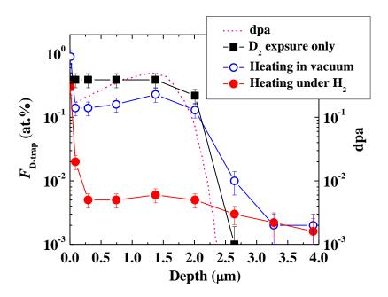
Fig. 4 Damage and D depth profiles in recrystallized W irradiated with 20 MeV W ions to 0.5 dpa. The D profiles were measured after exposure to  $D_2$  gas at 673 K and 0.1 MPa, and subsequent heating in a vacuum or under  $H_2$  atmosphere at 673 K for 10 h.
