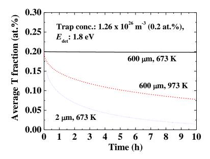
Fig. 6 Change in average T fraction throughout the thickness of n-irradiated W evaluated by using the TMAP4 program. The thickness of W was adjusted to 2 or 600  $\mu$ m. Trap concentration was assumed to be uniform at  $1.26 \times 10^{26}$  m<sup>-3</sup> (0.2 at.%) throughout the thickness. The initial  $\theta_t$  and  $E_{det}$  were adjusted to unity and 1.8 eV, respectively.
