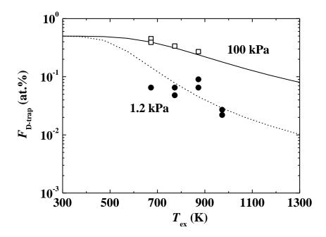
Fig. 2 Correlation between  $F_{\text{D-trap}}$  at damage peak and  $T_{\text{ex}}$  in W specimens irradiated with 20 MeV W ions to 0.5 dpa after exposure to  $D_2$  gas at P=1.2 kPa (filled circles) or 100 kPa (open squares). Solid and dashed lines are evaluated with Eq. (4) with H solubility reported by Frauenfelder [20] and  $E_{\text{bin}}=1.4$  eV.
