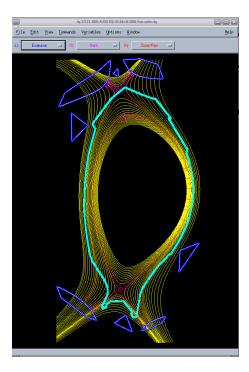
Fig. 4. Using the DivGeo geometry GUI to set up parameters for the CARRE 2 run shown in figure 2. Cyan=real device geometry, blue=virtual geometry
