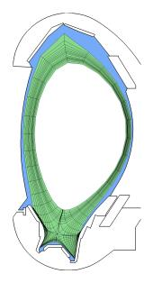
Fig. 1. The standard simulation domain for the SOLPS 5 covers the SOL (green). The region up to the wall (blue) is not covered.
