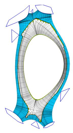
Fig. 2. Grid generation for a disconnected double null case, with the upper x-point outside of the vacuum vessel. Virtual geometry structures are shown in cyan, real geometry structures are black. Cell colors: white = internal, green = boundary, blue = external.
