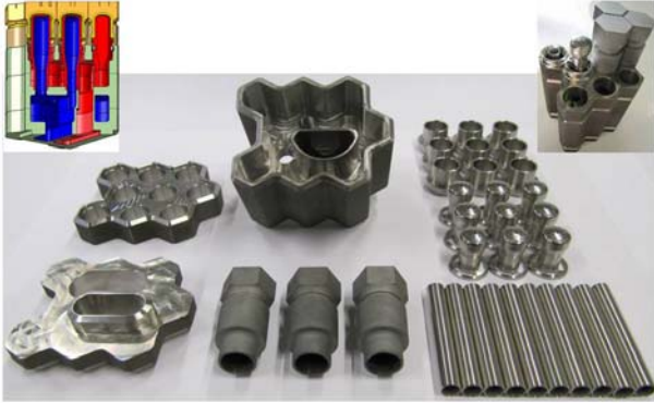
Fig.3 concept and individual parts of the 9-finger module of He-cooled divertor module developed at KIT [12].
